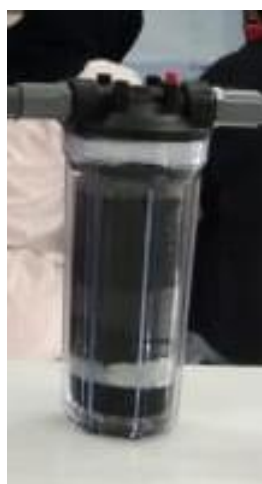
Figure 1. The Catridge Filter with Activated Charcoal
