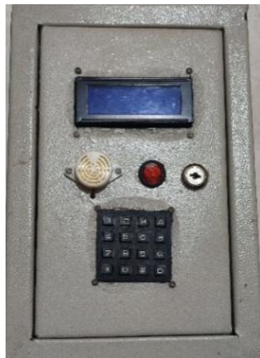
Figure 4. Final Prototype Of The Single-Phase Electrical Protection System.
