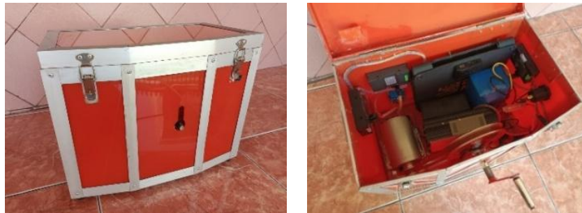
Fig. 2. Implementation of the Hybrid Portable Emergency Energy Box
