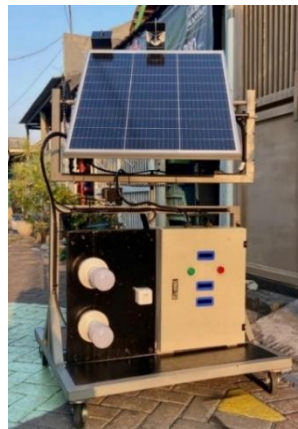
Figure 5. Overall View Results of the Dual-Axis Solar Tracking Source : Personal Documents
