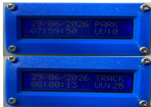
Figure 8. LCD Display to Monitor Tracking Operations Source : Personal Documents
