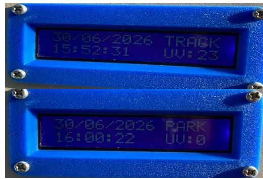
Figure 9. LCD Display to Monitor Parking Operations Source : Personal Documents
