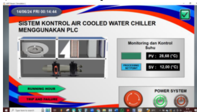
Gambar 14 : Halaman On / Off Sistem Kontrol, Input Set Point, Serta Status Monitoring
